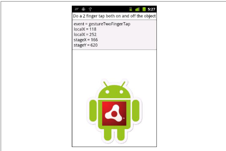
Figure 4-10. A two-finger tap on an image object
